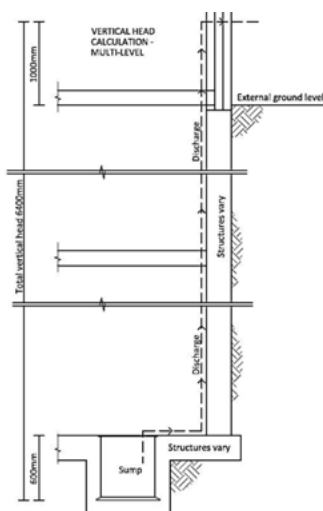
Example of multiple level basement depicting discharge pipe – vertical head calculations
