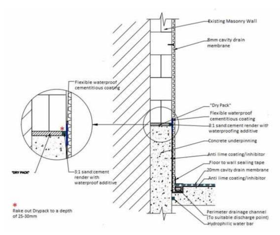
Free lime and mineral salts can leach from dry pack and new concrete and pose the potential risk of failure to Type C systems. As free lime leaches from the new construction by groundwater ingress, it deposits itself within the drainage cavity, (behind and underneath membranes) and particularly within the sump chamber and around the sump pumps. Thus, blocking free drainage, potentially causing pump failure and therefore failure of the system.
