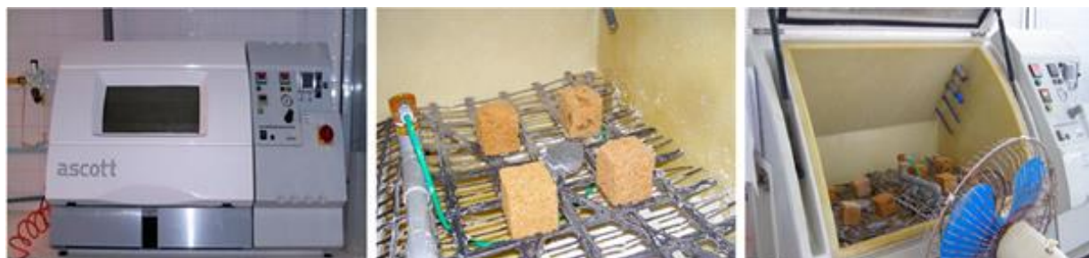
Figure 4. Marine aerosol (sodium chloride) accelerated aging test. (a) Salt Spray Corrosion Test Chamber; (b) Drying process without ventilation; (c) Drying process accelerated by ventilation (fan).
