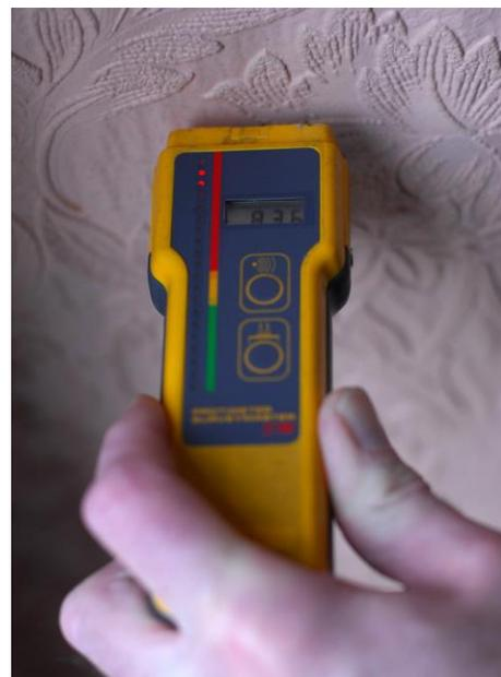
Moisture meters and other methods of determining the presence of moisture in building materials cannot differentiate between dampness from one source and that from another. It is therefore necessary to consider all potential causes of dampness before arriving at a conclusion.
