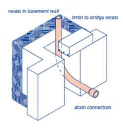
Where services penetrating the system are unavoidable the design and detailing to seal such elements should ensure that they are watertight and durable and suitably situated to allow for such works to be carried out (having them too close together can be problematic for detailing). In all cases details that penetrate a waterproofing system should be detailed and installed in accordance with the relevant manufacturer's guidelines.
