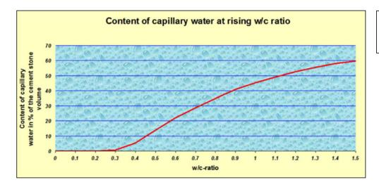
Two fold increase in capillaries from 0.5 to 0.6 W/C Ratio
