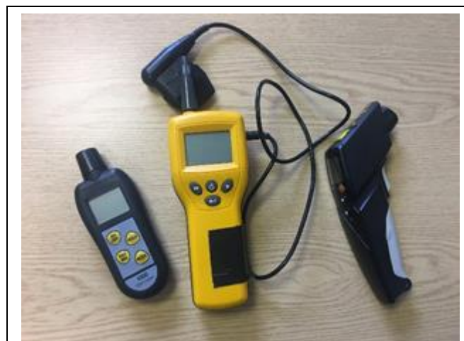
Fig 1. Selection of some of the tools a surveyor should have at their disposal, such as hygrometer, moisture meter and surface thermometer
